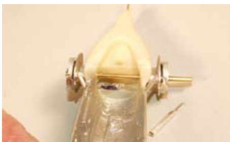
5. Spring cut in half to make fitting of rear suspension easier
