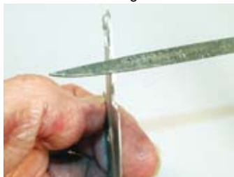
Just a few small mould lines to clean up
