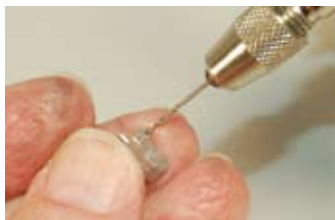
Several holes to be drilled with dimples marking the centre points
