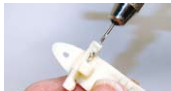
Opening up rear axle mounting to allow adjustment
