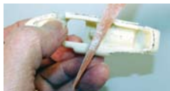
Emery board used to clean off mould lines
