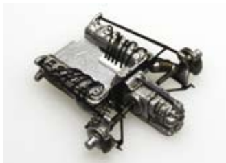
Completed drive-train assembly. Note plug wiring added to heads and ending out of sight on top of engine
