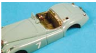
Coaming filed off the seat back and door panel to refit tonneau
