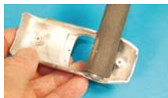
Excellent castings with just a few mould lines to remove, here on the insides of the wheel arches
