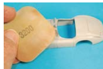
First primer reveals a few small blemishes, sanded smooth and filled with more primer
